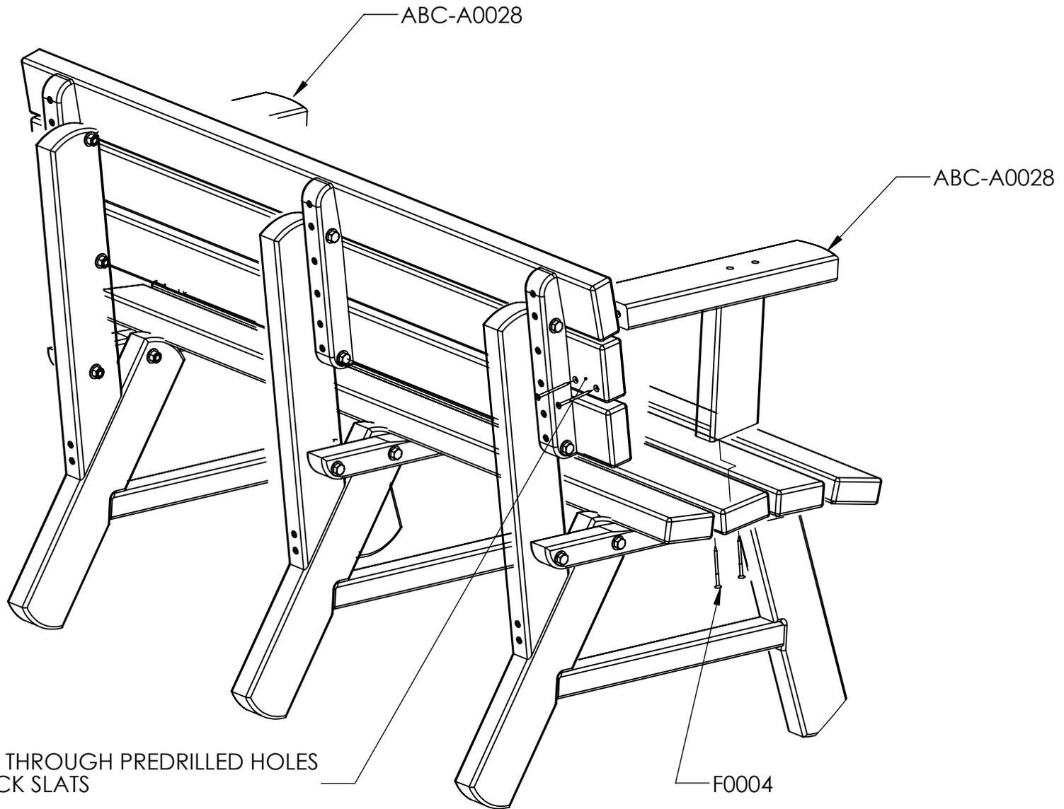
ATTACH ARMREST THROUGH PREDRILLED HOLES
