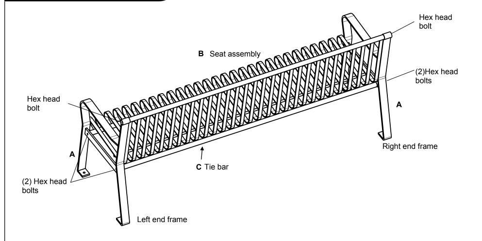
Step 3: Insert the tie bar into the back, bottom of each bench end. Screw in bolts enough to hold securely, but do not tighten. Make sure that the bench is square and level. Tighten all loose bolts to secure.
